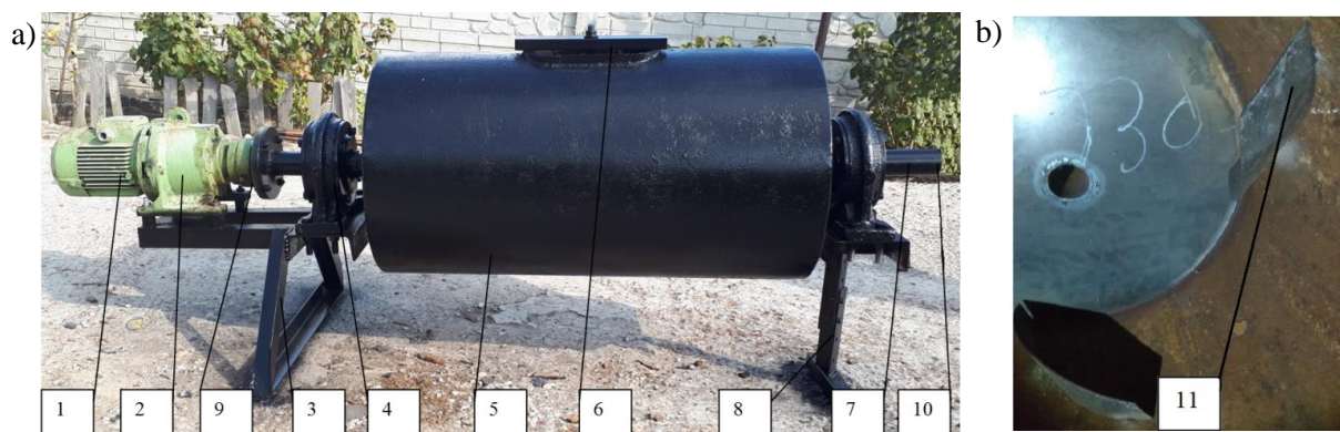
Fig. 1. Pilot plant [18]: a – physical appearance; b – stationary fixed blades
